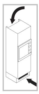
Check from time to time that the ventilation openings located on the back and underneath the cabinet which houses the appliance are free from any obstructions or dust. Contact your Service Assistance Centre for any necessary controls of the ventilation openings found on the back of the appliance.
